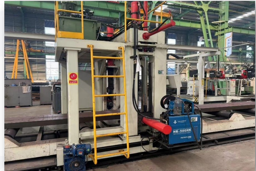
Box girder assembly machine
