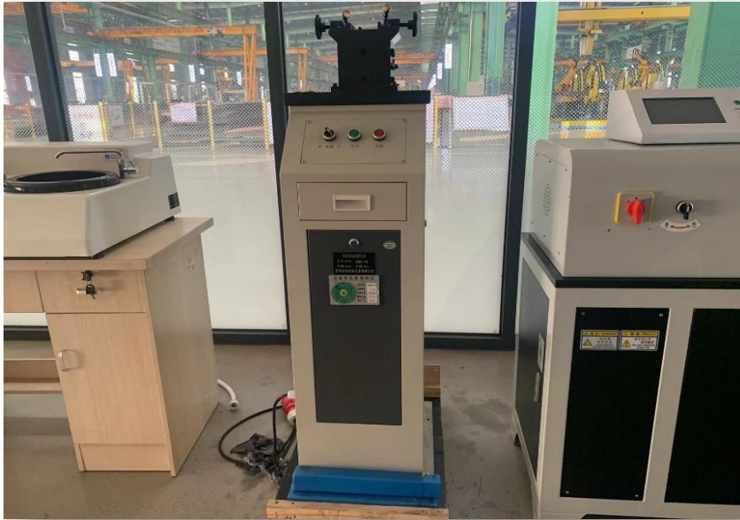
Impact sample notched hydraulic broaching machine
