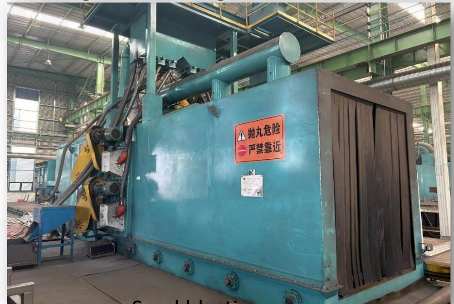
Sand blasting room
