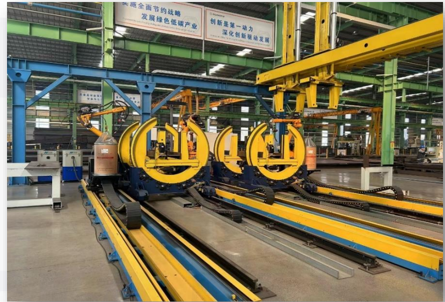
Robot Welding Station
