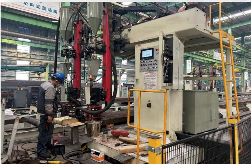
Box girder SAW machine
