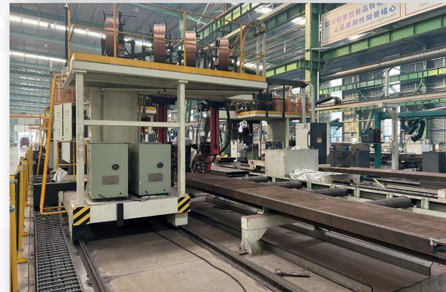
Box girder SAW machine
