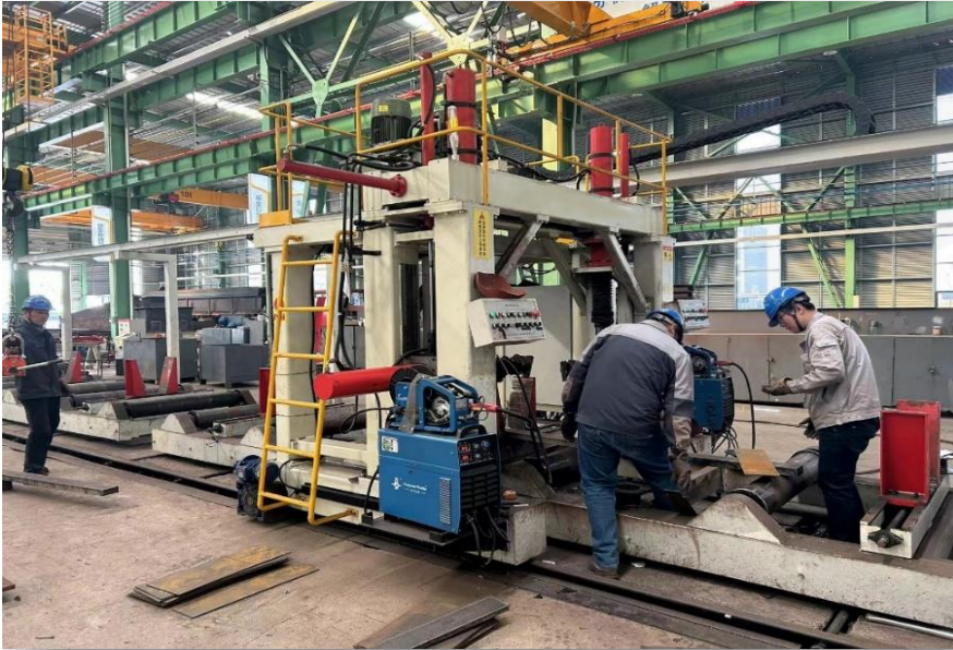
Box girder assembly machine
