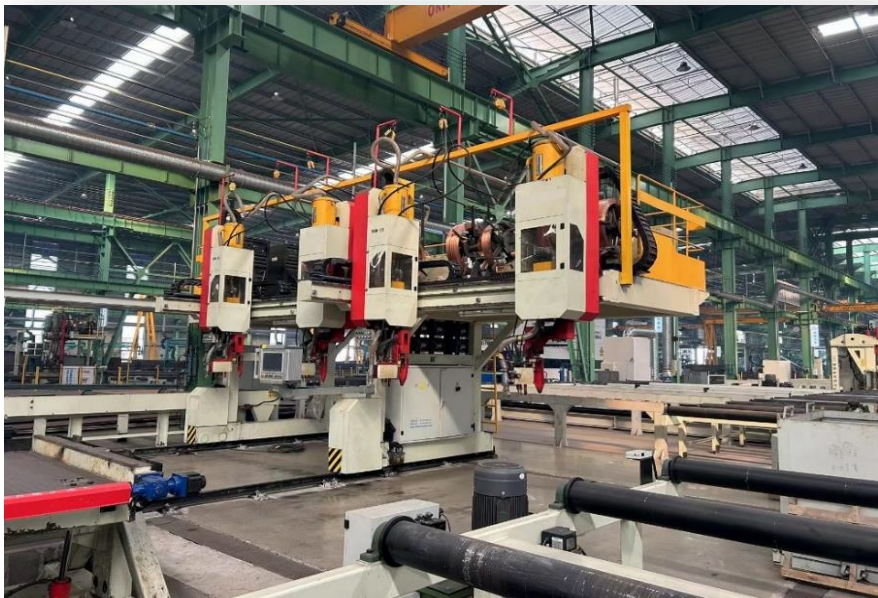
H-Beam Intelligent production line
