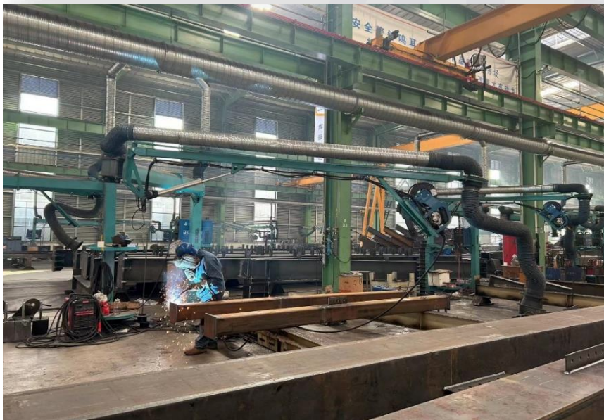
Welding fume extraction arm
